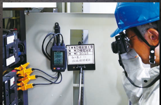
Display phase sequence, 3-phase voltage Use as-is in work certification photos
