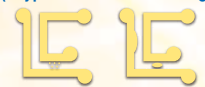
Impurity or void in insulating material Narrowing of gaps due to abnormal pattern shape
