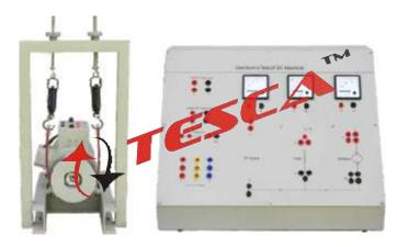
46602 Swinburn's Test of DC Machine is an important training system for Electrical Laboratories. It can be aptly employed for understanding the fundamental concepts and functioning of DC Motor. Swinburn's Test is the method through which losses are measured separately and efficiency at any desired load can be predetermined.
