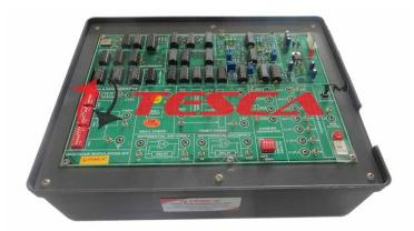
Order Code-40623 is an Advance Digital Communication Trainer System that helps one under stand various Digital Modulation and Demodulation Techniques. Various functional block diagrams are provided on-board as an aid for Teaching/Training. These Kits are provided with various Test Points to visualize the signals on Oscilloscopes.
