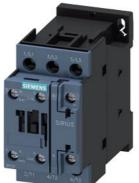
power contactor, AC-3e/AC-3, 9 A, 4 kW / 400 V, 3-pole, 230 V AC, 50/60 Hz, auxiliary contacts: 1 NO + 1 NC, screw terminal
