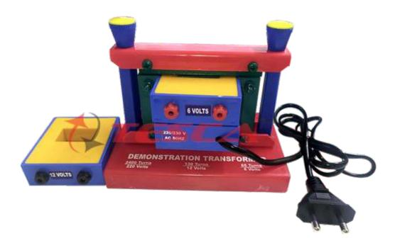
This apparatus has been designed primarily for demonstration of the basic principles of the a.c. transformer. The various coils and cores will also serve as the basis of many experiments in electromagnetism, using either direct or alternating current.
