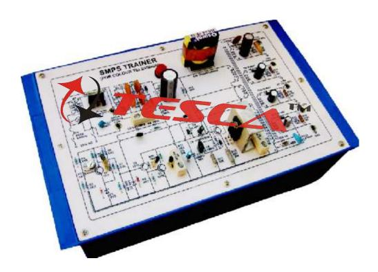
Experimental Training Board has been designed specifically for the study of Switching Mode Power Supply (SMPS) for Colour Television. The training board is assembled on enlarged PCB with different test points to observe waveforms and voltages. Now a days Switching Mode Power Supplies are extensively used in Colour Televisions i.e. 14" & 20" CTV's.
