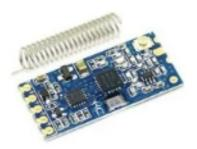
**Description-**HC-12 wireless RF UART communication module is a new generation of multichannel embedded wireless data transmission module. The Radio frequency of 433.4 – 473.0MHz, can be setting a communication channel, step is 400kHz, a total of 100 channels. The module maximum transmit power is 100mW (20dBm), and -116dBm receiver sensitivity air of the 5000bps baud rate, communication distance about 500 meters.
