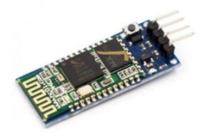
**Description-**HC-05 4 Pin Wireless Serial Bluetooth Module is a Bluetooth module for use with any microcontroller. It uses the UART protocol to make it easy to send and receive data wirelessly.
