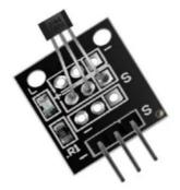
**Description-** The A3144 Hall Effect Sensor Magnet Detector Switch for Arduino is a switch that will turn on/off in the presence of a magnetic field. If no magnetic field is present, the signal line of the sensor is HIGH (3.5 V). If a magnetic field is presented to the sensor, the signal line goes LOW, at the same time the LED on the sensor lights up
