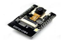
**Description-** The Esp32-Cam Has A Very Competitive Small-Size Camera Module That Can Operate Independently As A Minimum System.
