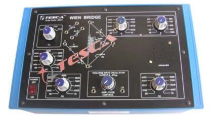
Experimental Training Board has been designed specifically for the study of Wien Bridge and by which one can evaluate the unknown value of capacitance.
