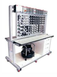
Double-Sided Mobile Workstation Allows The Assembly And Operation Of The Various Components Without The Use Of Tools (components Equipped With Quick Assembly System) The Workstation Must Be Equipped With:
