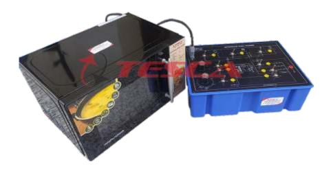
The 10953 Microwave Trainer Kit is an ideal training equipment to teach the operation of Microwave Oven. The complete Block of Microwave Oven is printed on single PCB for easy understanding of function of different blocks. Test points allow the analysis and monitoring of the signals in different sections. By using the fault simulation method, it is possible to introduce the most common breakdown and their rectification.
