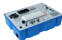
52072A Arduino Development Board
