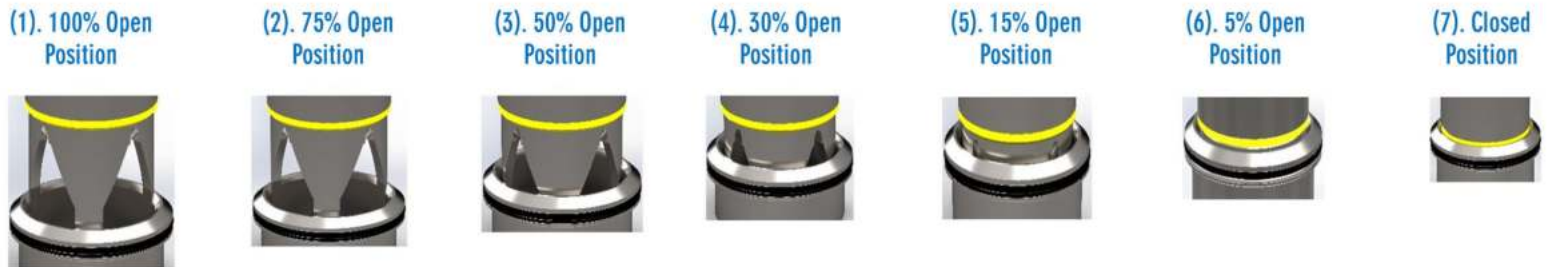
Figure 1: V-Port Open Positions At Incremental Percentages
