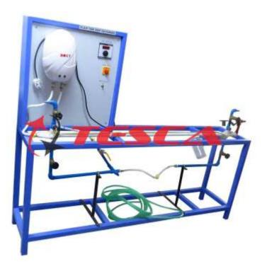
The apparatus consists of two concentric tubes. Inner tube consists of copper tube through which hot water flows. While the outer tube consists of GI pipe through which cold water flows. The arrangement enables the parallel and counter flow of the cold water. The inlet and outlet temperatures and the flow measurement enable to find out the heat exchanged LMTD, and effectiveness of the equipment.
